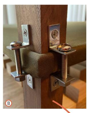
bolts and L brackets were a solution to having to attach the wood legs to fabric. this allowed the fabric to stretch and also did not create any cuts that would later rip.
