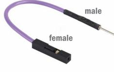
jumper wires connect everything to the breadboard and the bread board to the arduino.
